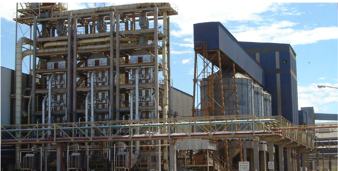
One of Terminal 6's crushing plants. Their milling capacity is 20,000 tons per day, and obtains the following by-products: Protein Flour, Crude Oil & Shell Pellets.
