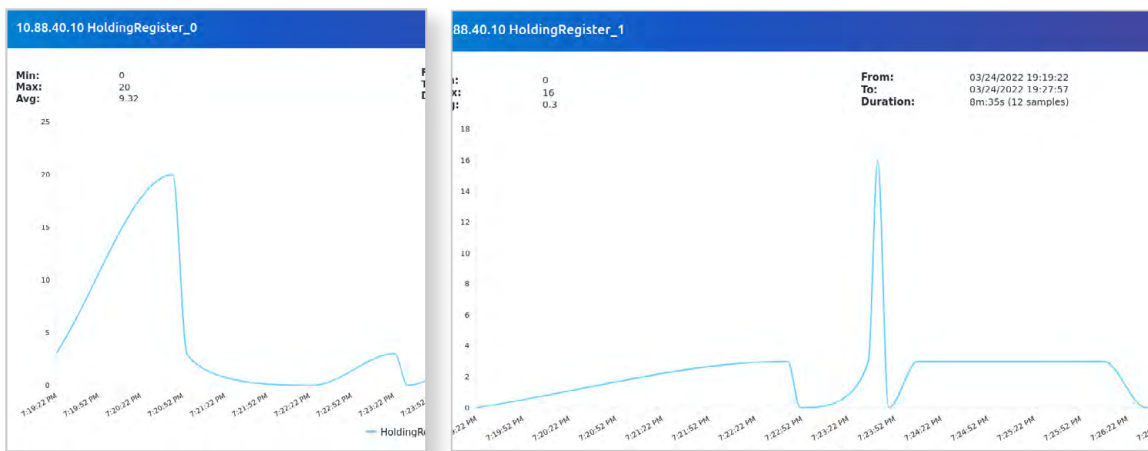
The SCADAfence Platform Value detects changes on a PLC, done from a compromised domain controller via the Modbus protocol.
